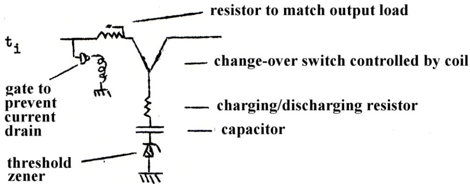
Of course, voltage levels and component values would need to be chosen carefully to be compatible with the logic circuit. With such a box it is fairly easy to construct output (2)
