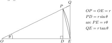
If  $\angle POD = \theta$  in radians, PE, the arc subtended by the angle  $\theta$ , is  $r\theta$  and  $r\theta > PD = r\sin\theta$ . Also,  $QE = r\tan\theta > r\theta > PD$ . So
