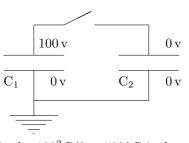
Initially the total energy in the system is the  $100^2C/2 = 5000C$  joules stored in C<sub>1</sub>. But when the circuit has settled down after the switch is closed, the energy is split between the two capacitors at  $50^2C/2$  joules each, making a total of 2500C joules. What has happened to the other 2500C joules?
