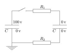
This is more or less precisely the circuit that was analysed in M500 246 by Mike Lewis. So I can just quote his final result. At time t after the switch is closed the current is
