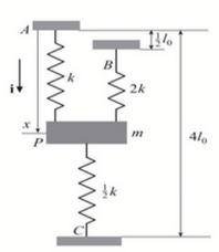
Model the block as a particle and the springs as model springs. Take the origin at A, and the unit vector i pointing vertically downwards. Let x be the displacement of P from A at time t.
