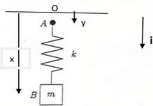
The vertical displacement at time t of the particle at B from the fixed point O is denoted by x(t), whereas the vertical displacement from O of the other end A of the spring is denoted by y(t), a known function of time. In the appropriate SI units the constants have the values m=1, k=4 and l=5, and the magnitude g of the acceleration due to gravity may be assumed to have the value 10. Throughout the question you should neglect any effects due to damping and air resistance.
